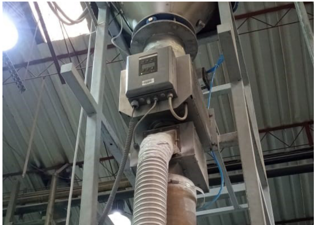
Metal separator RAPID VARIO-FS installed to protect a pelletizing extruder for PVC.
