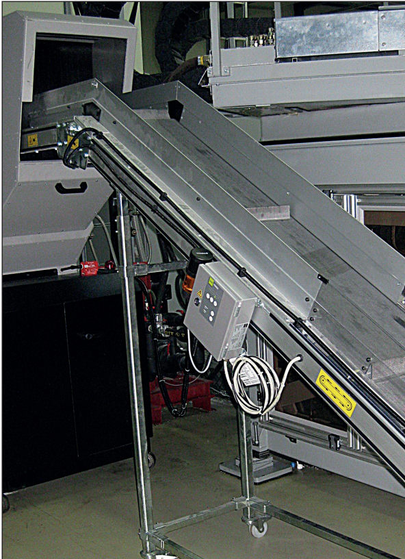
Installation example: Machinery protection. Plate type metal detector ELCON installed on the conveyor belt leading to the granulator. (old version)
